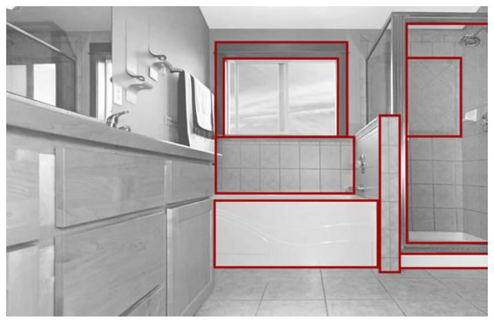
In one point perspective, surfaces that face the viewer appear as their true shape, without any distortion. They are drawn using primarily horizontal and vertical lines, as illustrated by the picture above.
